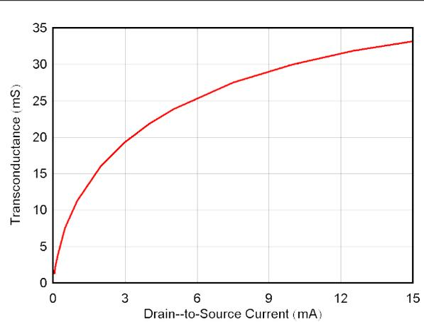
图 6-4. Common Source Transconductance vs Drain-to-Source Current
