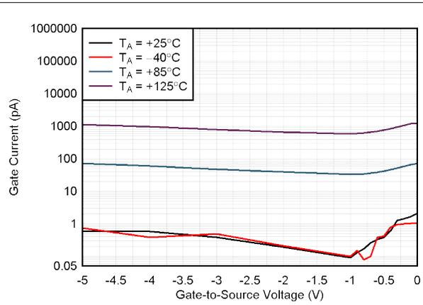
图 6-6. Gate Current vs Gate-to-Source Voltage
