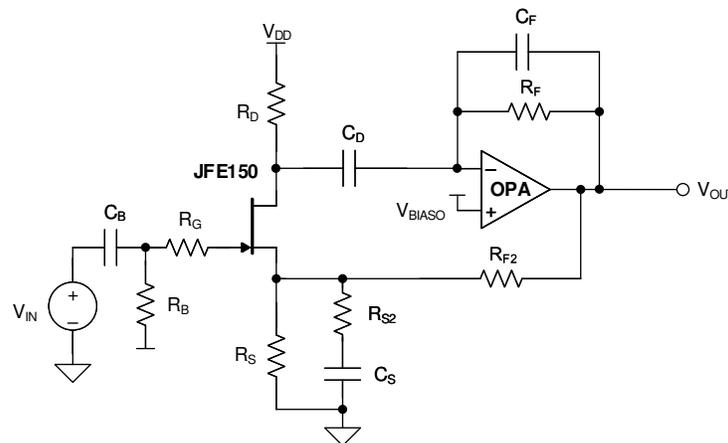
图 9-5. Low Noise, High Input Impedance Composite Amplifier
