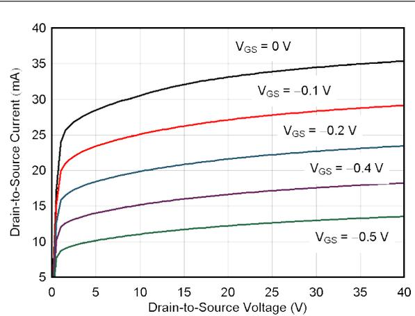
图 6-2. Drain-to-Source Current vs Drain-to-Source Voltage
