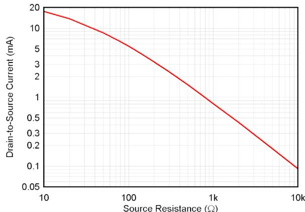
**图 9-3. Drain-to-Source Current vs  $R_S$ ,  $V_{DS} = 5 \text{ V}$**
