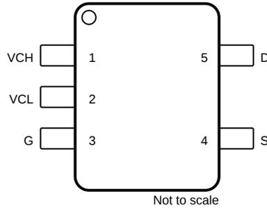
**图 5-1. DBV (5-Pin SOT-23, Preview) and DCK (5-Pin SC70) Packages, Top View**
