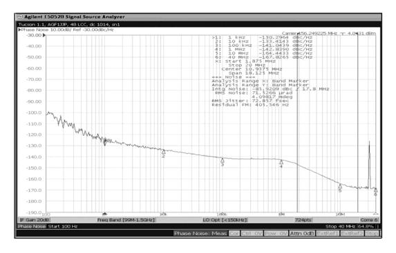
Figure 2. LVPECL Output (156.25MHz), 1.875MHz-20MHz Integration Bandwidth, 73fs Jitter, All Outputs Active
