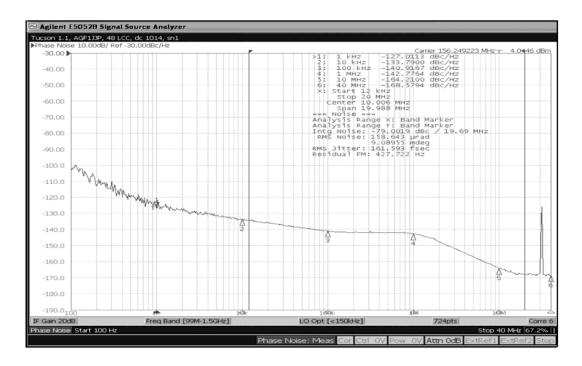
Figure 1. LVPECL Output (156.25MHz), 12kHz-20MHz Integration Bandwidth, 162fs Jitter, All Outputs Active
