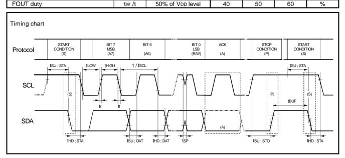
Caution: When accessing this device, all communication from transmitting the start condition to transmitting the stop condition after access **should be completed within 0.95 seconds**.
