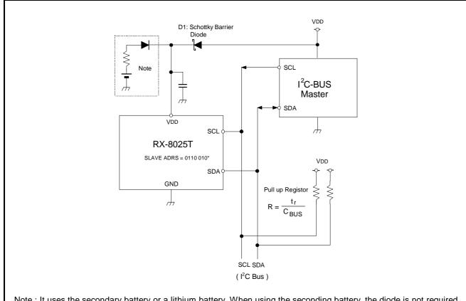
Note: It uses the secondary battery or a lithium battery. When using the seconding battery, the diode is not required.
