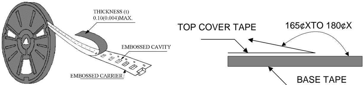
The force for peeling off cover tape is 10 grams in the arrow direction.
