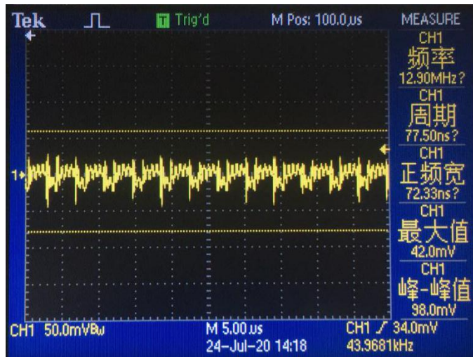
Noise (VIN = 48V, IO = 2.5A, 5 ~ 20MHz bandwidth)
